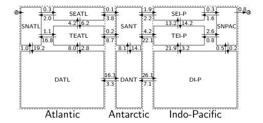
MBM model reservoir distribution, and water circulation scheme (fluxes in Sverdrup).
