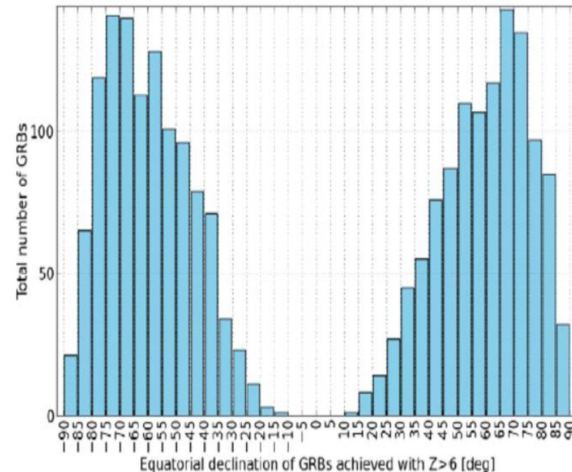
**Note:** Above results are not driven only by the SC agility model that provides a SC response time "average slew time" of 210sec but also due to the follow-up definition a.k.a a condition of finding a window of 7mins continuous exposure time. Even with a goal requirement in the SciRD/MRD of SC agility of 3 mins the compliance to this requirement for 100% of triggers is not believed to be feasible.
