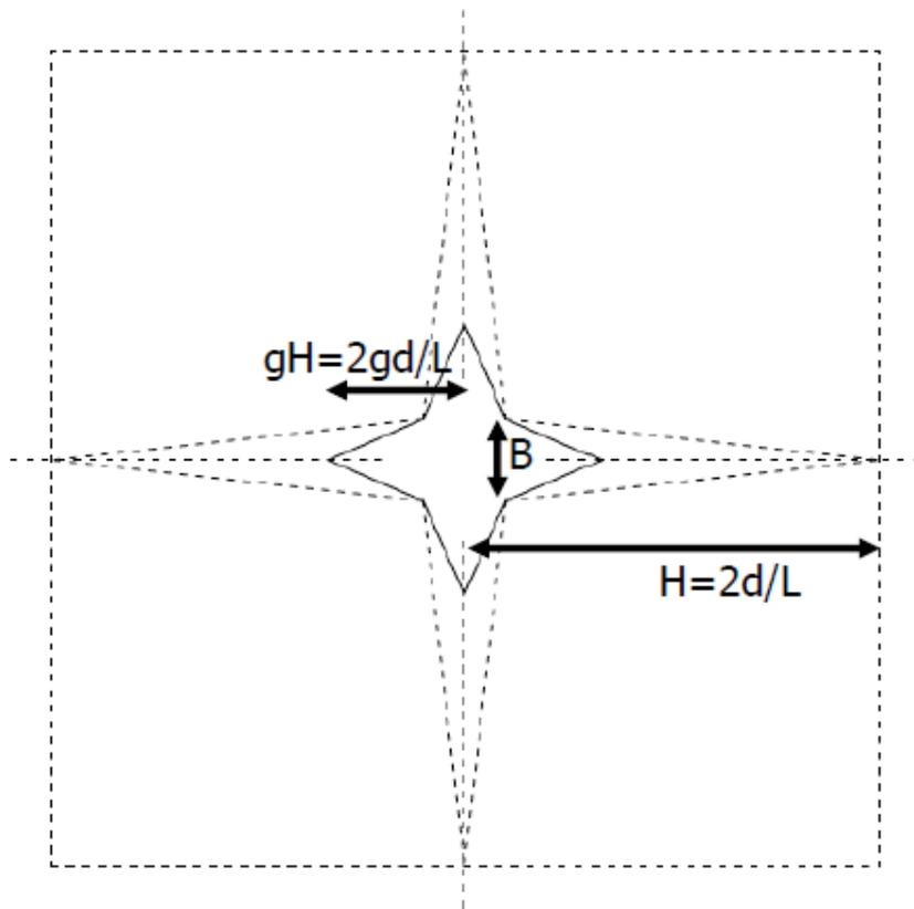
A conventional circular beam is not a good approximation to the PSF shape
