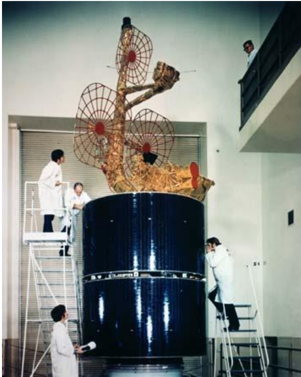
Figure 5.4: Left: a satellite of the Intelsat series during integration. These satellites were spin-stabilized. To generate the electrical power, the outer surface of the satellite is hence covered with solar cells. Right: schematic representation of a gyroscope.
