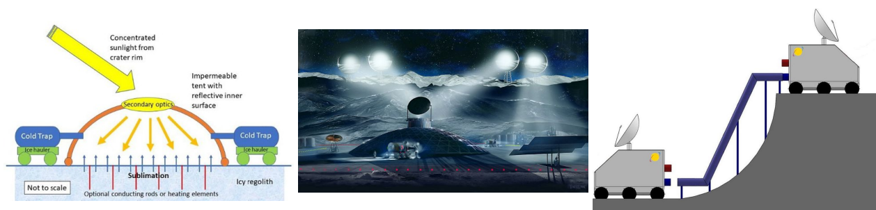
Figure 9.5: Left: schematic view of a mining tent for the extraction of water from the lunar soil. Middle: artist view of the power beaming used to concentrate sunlight onto a permanently shadowed extraction site. Right: schematic view of a robotic tanker combined with a pipeline near the crater wall to transport the extracted water. From Kornuta et al. (2019).
