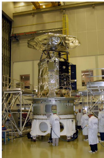
Figure 4.1: Integration of ESA's Herschel infrared space observatory in the cleanroom of ESTEC (Noordwijk).
