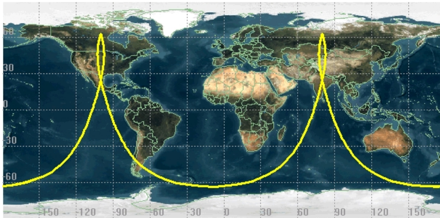
Figure 3.11: Projection of the Molniya orbit on the Earth. Since the orbital period is exactly half the rotation period of the Earth, only every second apogee occurs over Russia, the other one happens over North America.
