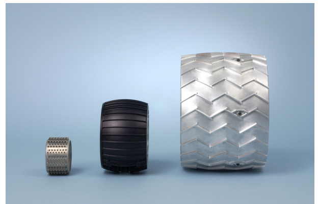
Figure 8.17: Left: an artist view of the Curiosity rover on Mars. Right: comparison between the wheels of the rovers Sojourner, Spirit and Curiosity.
