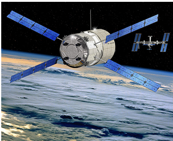
Figure 10.4: Left: artist impression of an Automated Transfer Vehicule approaching the ISS. Right: Schematic view of the ATV transfer orbit. Note that the various distances and radii are not to scale.
