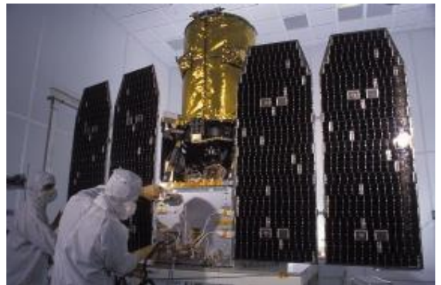
Figure 7.19: Left: the launch sequence of the GALEX satellite with the Pegasus rocket carried by the L-1011 aircraft. Right: the GALEX satellite during integration.
