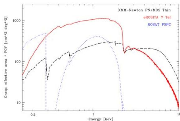
Figure 12: Grasp of eROSITA (red) in comparison
