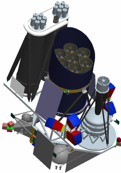
Figure 1: Preliminary SRG/eROSITA/Lobster/ART-XC/SXC spacecraft on (without solar panels).
