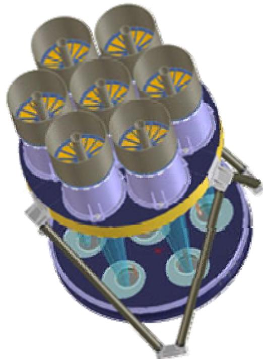
Figure 7: The seven mirror modules with the baffles in front and the seven cameras at the rear end of the optical bench. Total length of the telescope is <2,600 mm, the diameter is ~1,300mm.
