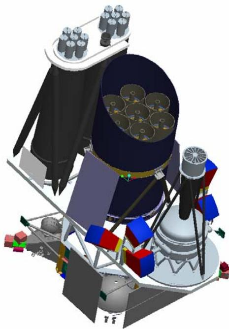
Figure 6: Spectrum-RG with the Navigator-spacecraft and the payload consisting of ART-XC, eROSITA, SXC (from left to right) and 5 modules of LOBSTER.
