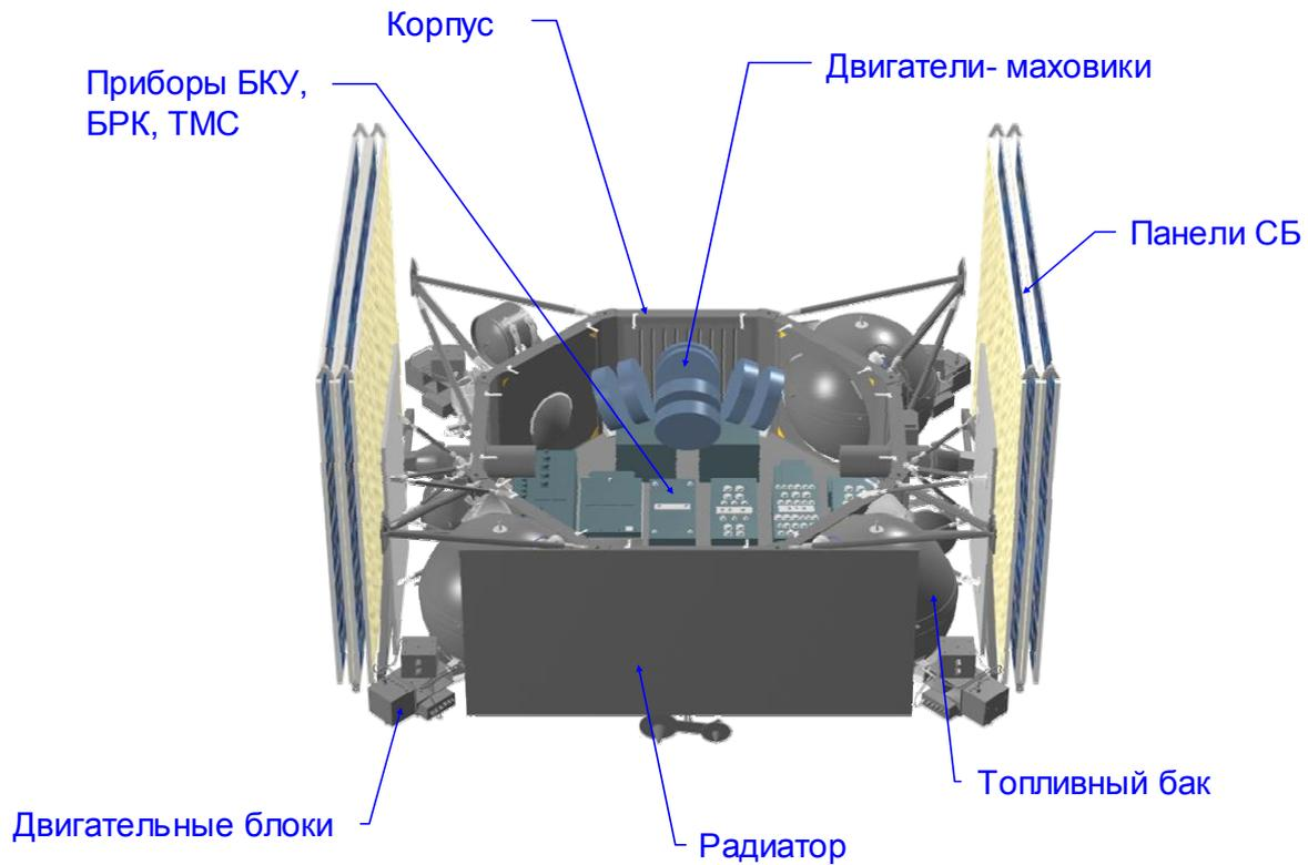
Figure 16: Schematic view of Navigator
