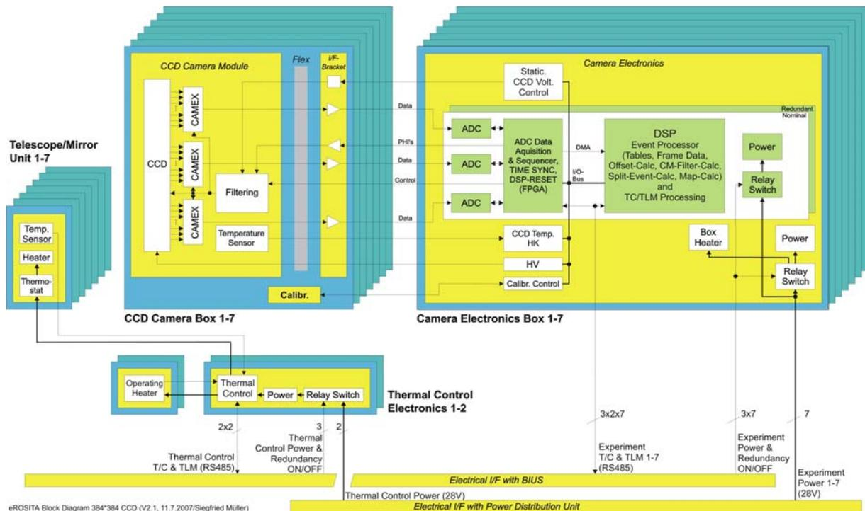
Figure 10: Scheme of the Camera Electronics. Each camera has its own (but identical) electronics. The critical part of the electronics (ADC, FPGA, DSP) is (cold) redundant. An 8<sup>th</sup> electronics box is for thermal control of the instrument.
