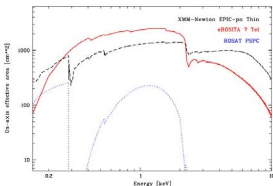
Figure 11: On-axis effective area of eROSITA (red)
