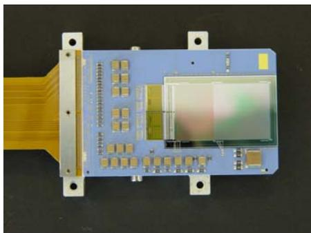
Figure 8: eROSITA CCD-Module. The CCD with its image area ( $3 \times 3$  cm<sup>2</sup>) and the slightly smaller frame store area (left) is connected via 384 bond wires with three CAMEX read out chips. They are mounted, together with the (passive) front end electronics, on a ceramic printed circuit board (blue). The flexlead on the left connects the CCD-Module with the experiment electronics. Shown is the older  $3 \times 3$  cm<sup>2</sup> version with  $256 \times 256$  pixel.
