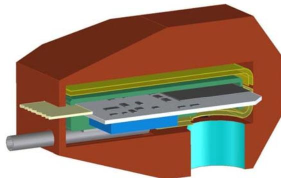
Figure 9: Schematic representation of the eROSITA Camera with the (warm) Cu-proton shield (brown), the thermal insulation (yellow), the housing (cold, green), and the CCD-Module (grey) which is thermally connected to heatpipes by a Ti-block (blue). An additional graded shield (magenta) suppresses fluorescent X-rays generated in the housing and leading to an enhanced background.
